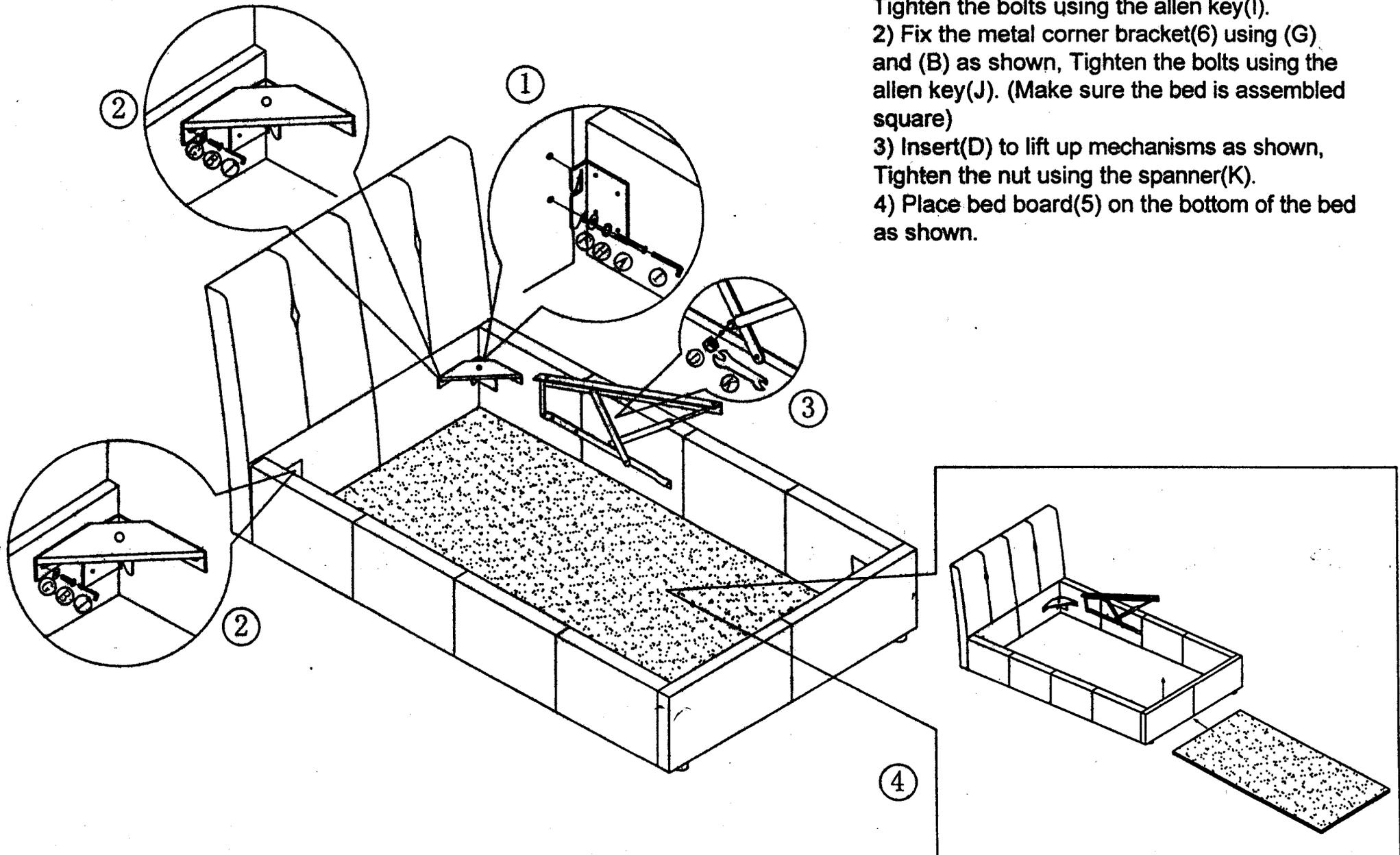
5) Fix the metal frame base(4) to the lift up mechanisms using(E),(G) and(C) as shown. Tighten the fitting using the allen key(J) and spanner(K).
